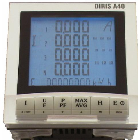
A multi-function panel mounting energy meter the **A40** will measure energy in 4 quadrants plus current and voltage harmonics. This meter provides more than just energy consumption information on its display. User configurable the multi-line, back-lit liquid crystal display will provide simultaneously four measurements (e.g. phases and total) plus bar graphs for each phase current.
